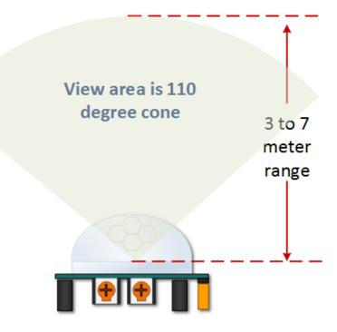
The device will detect motion inside a 110 degree cone with a range of 3 to 7 meters.
