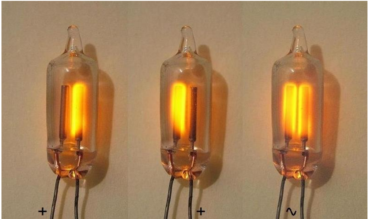
+DC (left), -DC (center), AC (right) supplied to Neon lamps
