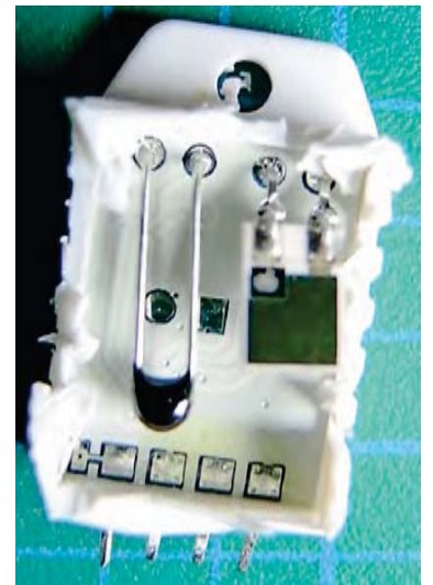
Fig.6 (right): the sensor module with the top of the case removed. The bead type sensor is an NTC thermistor and to its right is the capacitive humidity sensor.*
